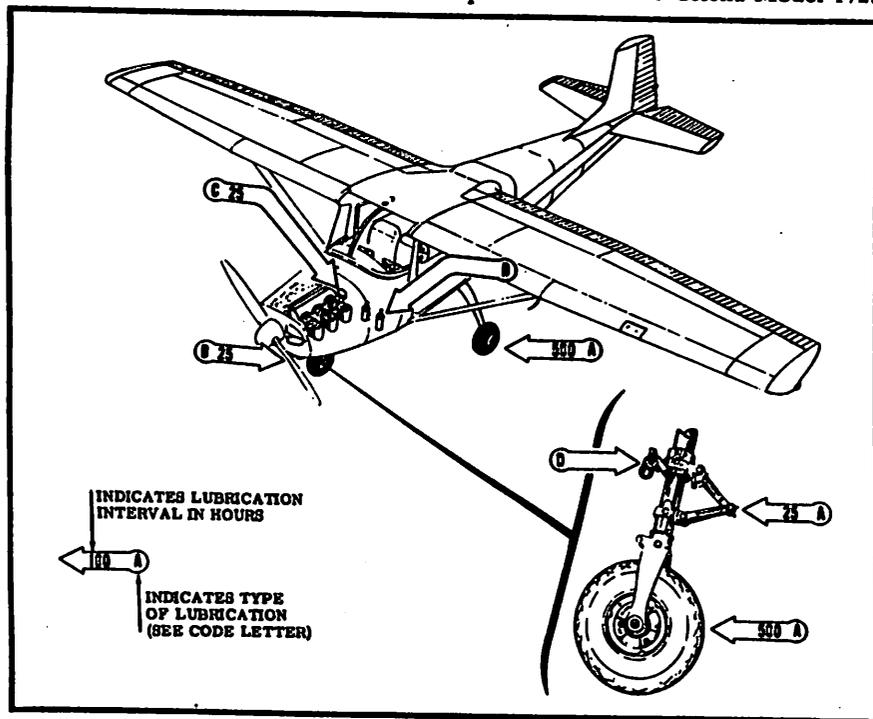
Figure 20. Lubrication Diagram
