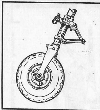
The steerable nose wheel is mounted on an air-oil shock strut which incorporates a shimmy dampener to assure smooth operation. This nose gear makes ground handling, taxiing, and landing both easier and smoother.
