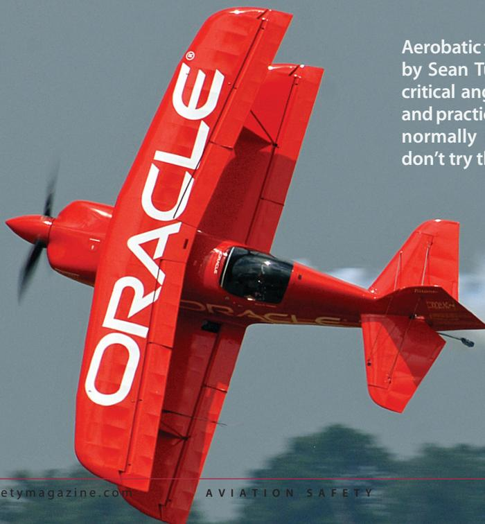
Aerobatic flight of the sort demonstrated here by Sean Tucker avoids exceeding the wing’s critical angle of attack through skill, training and practice. Having power in excess of what’s normally needed doesn’t hurt, either. Just don’t try this at home without some training.
